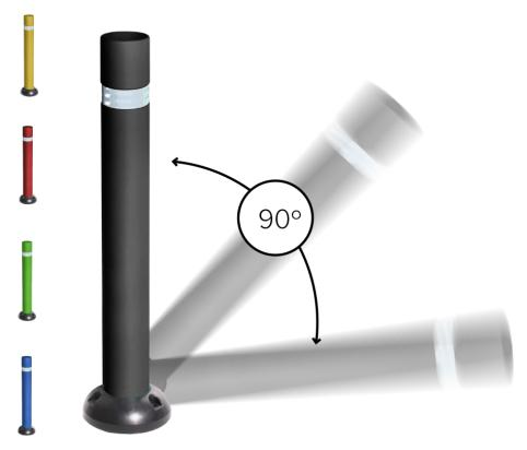
Bollard made of flexible black polyurethane resistant to UV rays with reflective band. With base plate for a bolt-on installation Manufactured in fixed and removable version with polyurethane or stainless steel base. Exceeds a flexion of 1500 cycles at 45° and 50 cycles at 90°, without damage.
