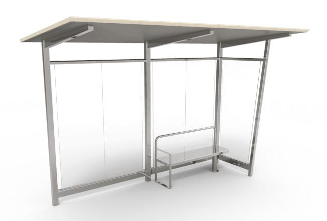
Bus shelter with pillars and bench made of bright polished AISI-304 stainless steel. Roof panel with three 80 x 80m support pillars for its fixing, with brackets and horizontal profiles for glass enclosure. Galvanised and pre-lacquered injected polyurethane roof. Laminated safety glass. Supplied in kit form, with accessories and assembly
