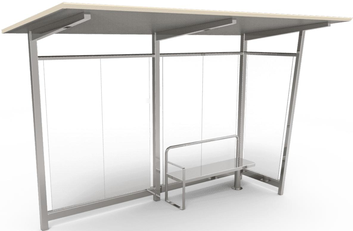
Bus shelter with pillars and bench made of bright polished AISI-304 stainless steel. Roof panel with three 80 x 80mm support pillars for its fixing, with brackets and horizontal profiles for glass enclosure. Galvanised and pre-lacquered injected polyurethane roof. Laminated safety glass. Supplied in kit form, with accessories and assembly instructions. Recommended anchoring: embedded in the ground.
