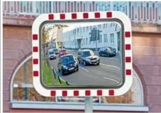
The **DURABEL LITE IceFree** Stainless Steel mirror is a low cost alternative to our DURABEL IceFree mirror, but retains the tried and tested thermo-gel system which controls the surface temperature of the mirror based on the actual ambient temperature. This system prevents the formation of condense and ice on the mirror surface down to -20°C.
