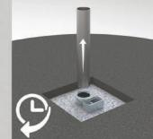
Replace pedestrian and side access covers. Re-instate finished surfacing.
