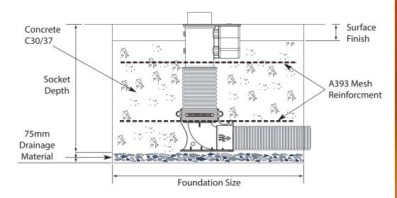
Foundation sizes shown here are based on loadings calculated using EN40-3-1:2000 for minimum post loadings and are guidelines only. For more detailed foundation sizing on specific site conditions contact your supplier.
