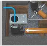
Insert and tighten levelling pole with bolts in the sidechamber of socket.
