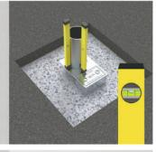
Remove levelling pole once concrete is set.
