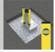
7 Remove levelling pole once concrete is set.
