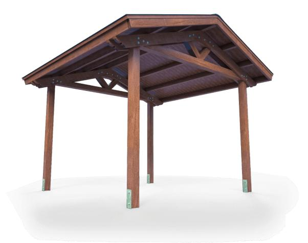
4000 x 4000 mm self-supporting gable roof pergola made from European Oregon (Douglas) pine. 120 x 120 mm pillars, 170 x 45 mm beams, 140 x 45 mm joists and 115 x 21 mm tongue-and-groove boards. Lasur coating, 100% natural vegetal oil- and resin-based varnish finish with a protective UV overcoat in golden oak colour.
